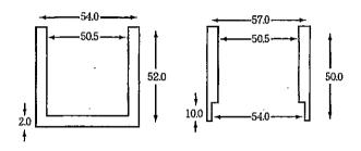
Fig. 3.01-2. Measuring vessel (left) and cap (right)
